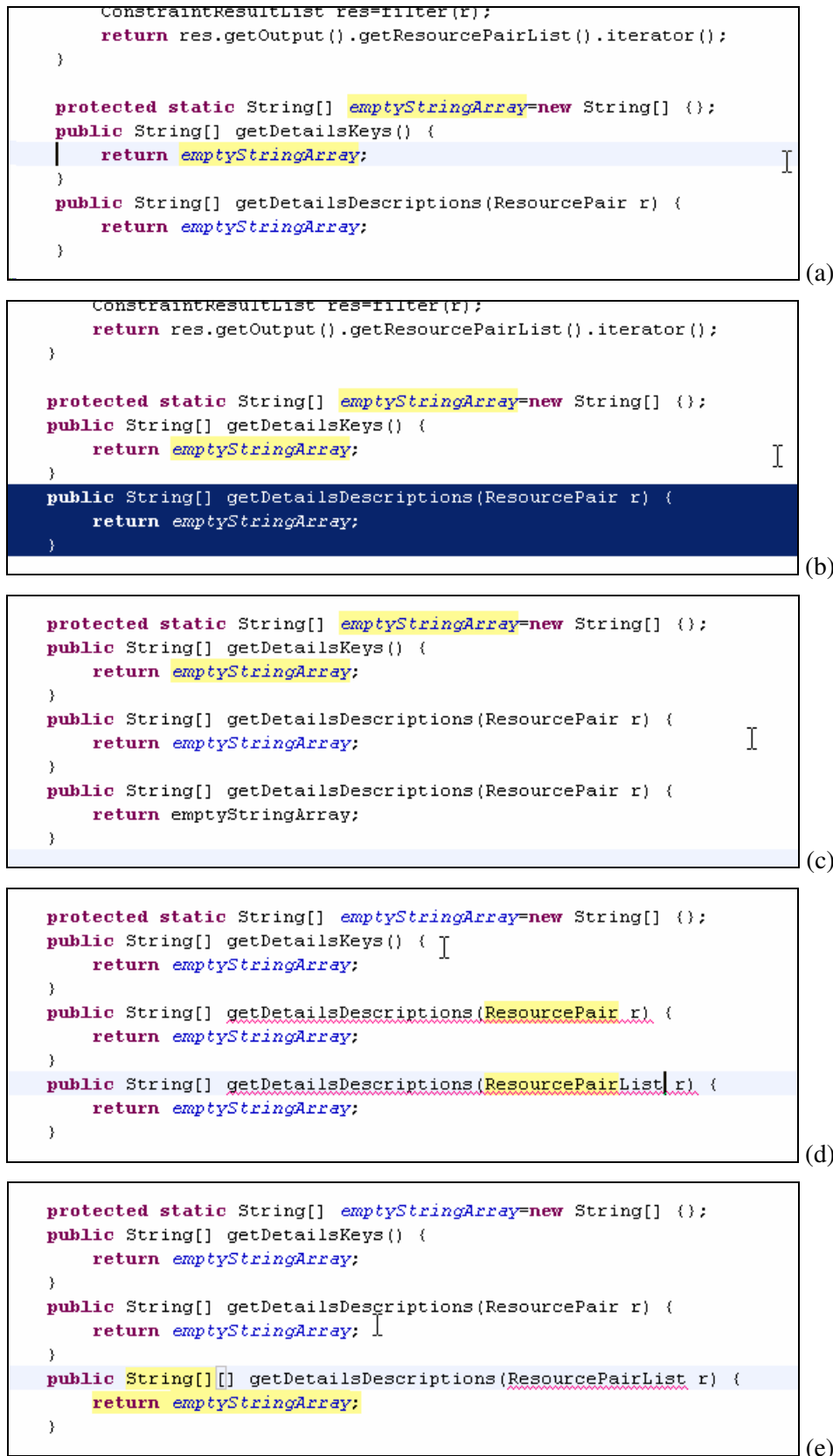
Figure 2 : Video stills from a Java code change: The programmer (a) positions cursor, (b) selects code part to be copied, (c) pastes code below the original, (d) changes parameter type, (e) changes return type. The editor (Eclipse) continuously highlights line of cursor (light grey), string matches of expression at position of cursor (yellow), and warnings/errors (curly underlining)
